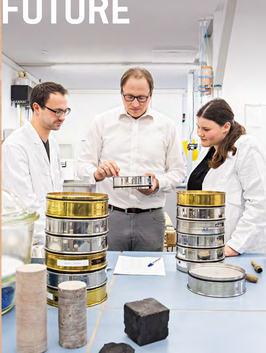
Prof. Christian Melchers (centre) with two of his students carrying out a sieve analysis in the lab at the Technische Hochschule Georg Agricola in Bochum.
